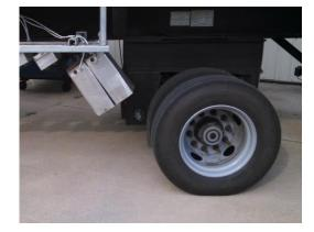
Right Wheel Path Laser RWD Left Wheel Path Image Based RWD (Shown)
