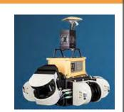
Mobile scanners are available with both TOF and Phase based scanners
