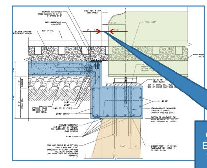
Gap Between Backwall and Girder End Designed at 3", then Revised to 10" during Bridge Seat Fabrication
